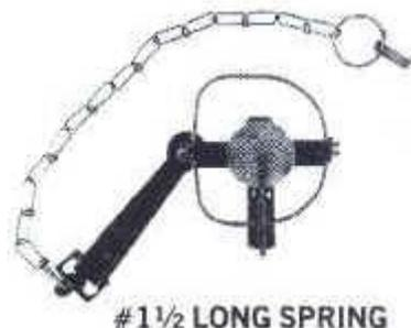
**This is a typical long spring leg hold trap.** The trap can be released by stepping down on the leaf spring to the left of the center pan. Double leaf springs will have springs on both sides -- step on both of them at once, as you would a coil spring trap.
